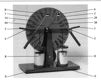
The Wimshurst Machine is a device for generating very high DC voltage.
