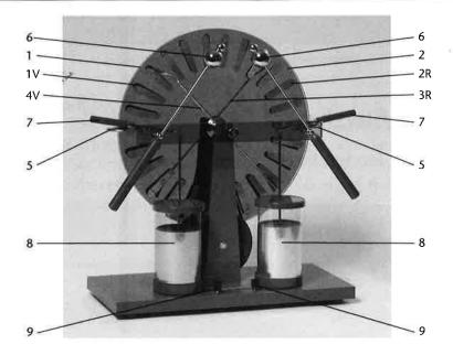
The Wimshurst Machine is a device for generating very high DC voltage.
